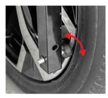
NOTE In order to prevent the screws from loosening when in use, the screws must be screwed inside as far as possible, preferably parallel to the other hole of the square tube.
